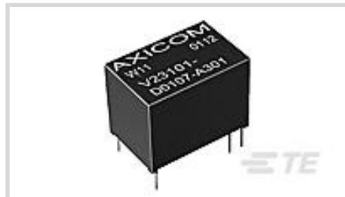
Relay & Contactor Type: **Reed Relay**Current Type: **DC**Coil Magnetic System: **Monostable**Contact Arrangement: **1 Form C SPDT-CO**Contact Current Rating: **3 A**
