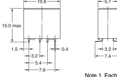
Note 1. Each value has a tolerance of  $\pm 0.3$  mm.
