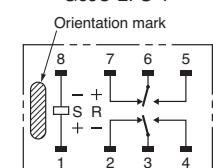
Note: Check carefully the coil polarity of the Relay.
