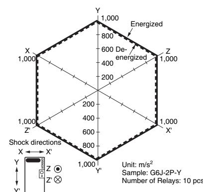
Test Conditions: Shock is applied in  $\pm X$ ,  $\pm Y$ , and  $\pm Z$  directions three times each with and without energizing the Relays to check the number of contact malfunctions.
