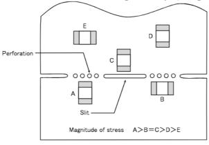
1-3. When PCB is split, the amount of mechanical stress on the capacitors can vary according to the method used. The following methods are listed in order from least stressful to most stressful: push-back, slit, V-grooving, and perforation. Thus, please consider the PCB, split methods as well as chip location.
