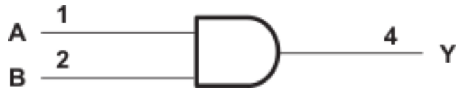
Logic Diagram (Positive Logic)
